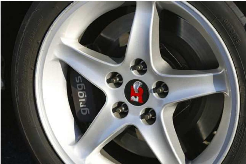
**Prior to a complete teardown and build as a street legal track car, Hicks ran Ford Performance's M2300K four-wheel disc brake kit. In the new configuration, the Cobra brakes were replaced by these Griggs/Sierra binders. The front uses a four-piston caliper with 13.5-inch two piece rotors, the rears are a four-piston 12.5-inch combo.**
