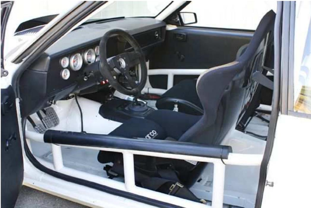
**The interior is all business, stripped of all unnecessary niceties. Highlights include a rally style roll cage, Sparco seats, Momo quick release steering wheel, and full array of Auto Meter gauges.**
