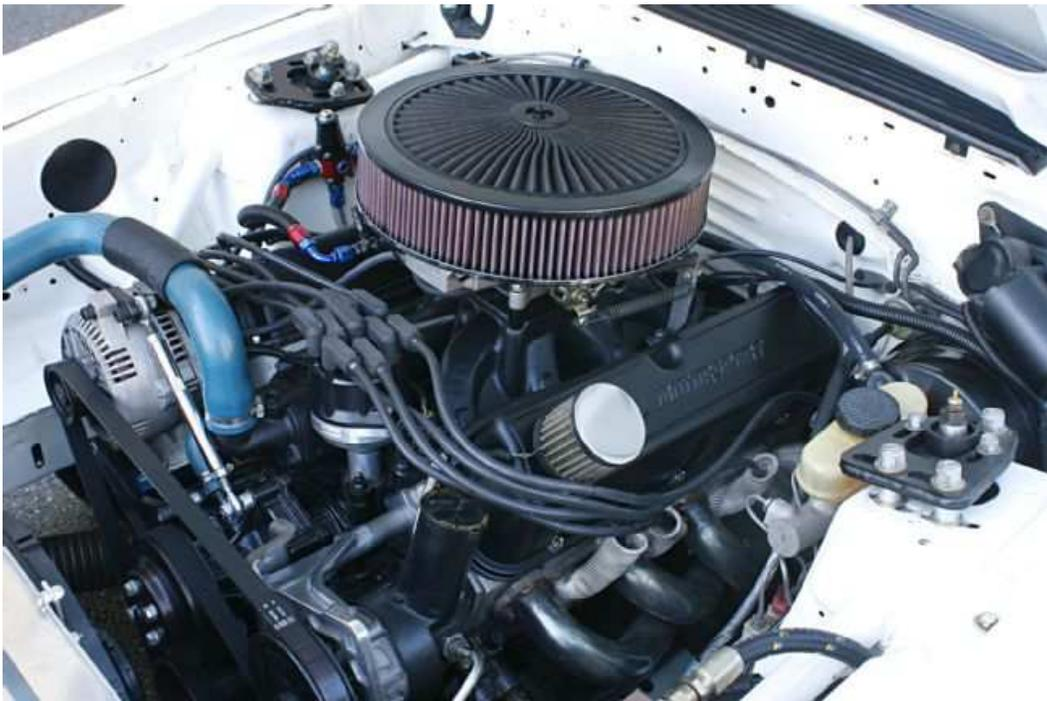
**Natural aspiration is the order of the day under the hood with a stout 331ci small-block. Horsepower is just shy of 400 to the rear wheels and provides consistently quick lap times. The stealth black approach is in sharp contrast to the white engine compartment.**
