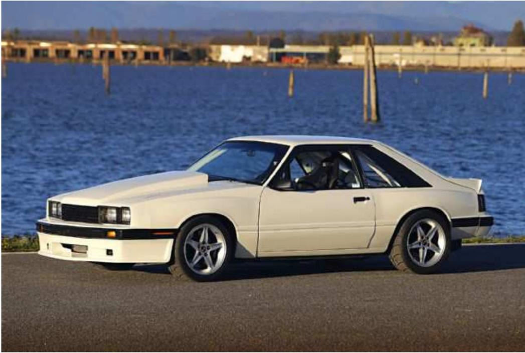
**Hicks' Capri is nicely finished in its original Polar White hue, courtesy of Chris White. The Sikkens paint products cover a blend of stock and aftermarket panels, the latter being an H.O. Fibertrends cowl hood and fiberglass hatch with lexan window. Lexan quarter windows are employed a well, helping achieve a total weight of 2,950 pounds sans driver.**
