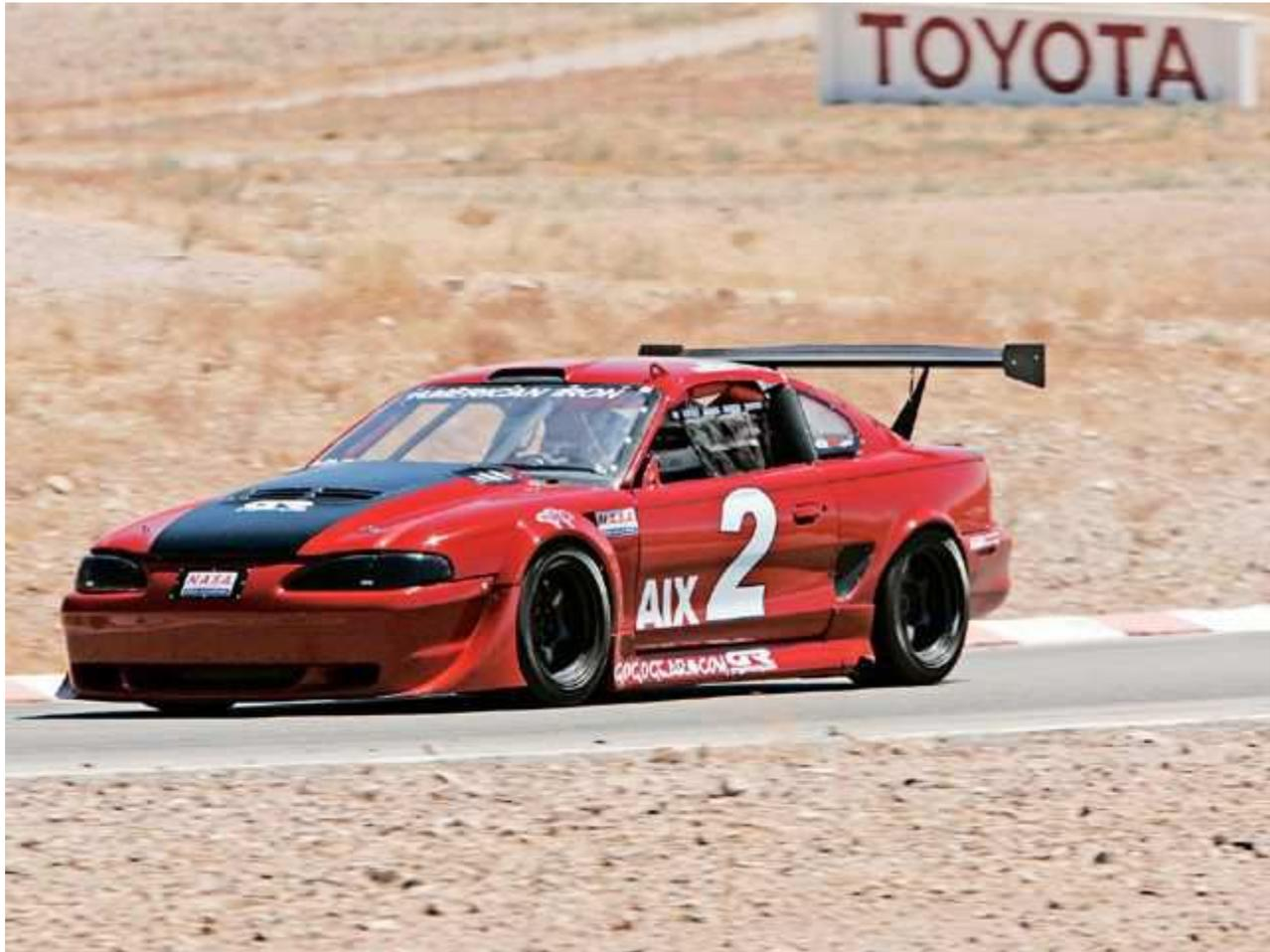
Some of those carbon parts are already in place, of course, especially at the front where the aerodynamics are aimed at increasing downforce. A Griggs nose and splitter, Tiger Racing front fenders, and dive planes (the swoopy tabs between the headlights and wheelwell) help plant the front end. In back, Ernesto categorizes his rear wing as "ultra wide" for maximum downforce. It isn't, he noted, the fastest car in a straight line, thanks to his high-downforce strategy.
